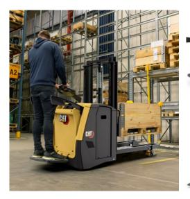
Double handling is achieved by placing one pallet Application-matched choices include a foldable load on the straddle legs and one on the forks. With this arrangement, the truck remains compact and is highly manoeuvrable even in tight spaces.
