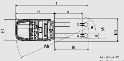
Ast = Wa-x+I6+200 Ast = Working aisle width Wa = Turning radius
