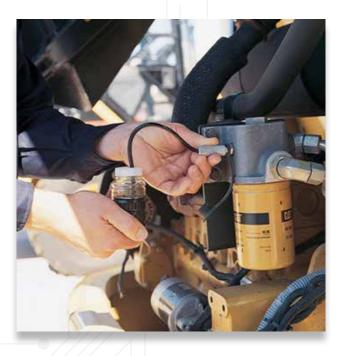
When it comes to oil testing, visual inspections are limited to the larger particles. We can spot early signs of damaging wear metals, the condition of your oil, overall particle analysis, and identify contaminants that hurt performance (water, fuel, glycol, dirt, etc). Our technicians perform comprehensive analysis on lubricated systems (engines, transmissions, hydraulics, final drives, differentials, gearboxes, compressors).
