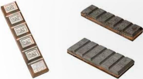
**Chocky Bars**, available in four shapes, feature a V-groove design that can be bent around a radius. They can be separated or modified in length. The inset of the Cat logo allows for the trapping of fine material in each section, extending the life of the wear material itself. Chocky bars come in four sizes.
