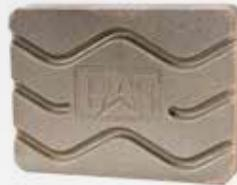
**Wear Blocks** feature a zigzag inset design that allows for material-on-material wear. They prevent channel wear common in parallel grooves, delivering extended life in extreme operations.
