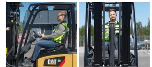
**The adjustable seat and steering column assure a perfect driving position for drivers of all sizes. Forward, downward and side views are excellent due to a specially designed free lift cylinder structure where hoses and chains are positioned to minimise obstacles to vision. Ergonomic controls include an adjustable armrest, with inbuilt fingertip levers, and a set of low-fatigue pedals.**
