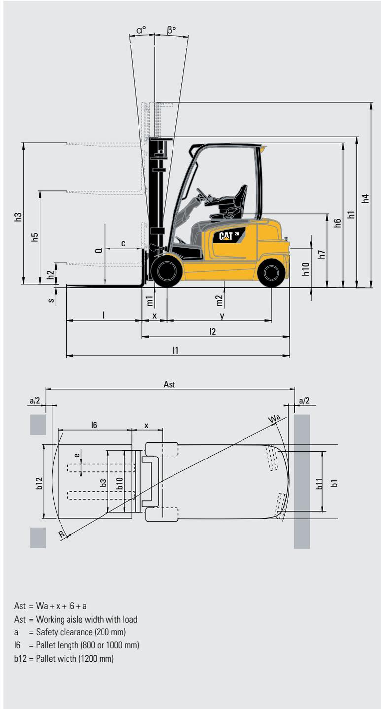
This specification sheet provides details of the standard truck specification in accordance with VDI Guideline 2198.
