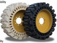
for a more cushioned ride than solid tires. They also serve as a means of absorbing shock that would have otherwise been transferred to the machine and the operator.
