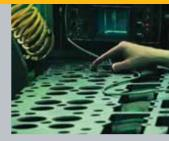
magna- fluxed to detect cracks, and inspected for other damage. The bottom deck is resurfaced to ensure a tight seal between the cylinder head and engine block to help prevent combustion gas and coolant leaks. All critical wear and sealing components are replaced with new Cat parts. Cat Reman Cylinder Heads are pressure tested for leaks before they leave the factory.
