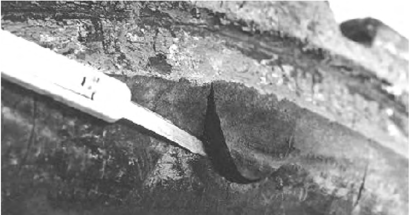
Illustration 6 Broken bead or damaged bead due to improper mounting
