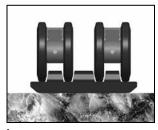
On a flat surface (Illus. 1), machine weight is spread through the roller wheels to the full ground contact area of the track. Minimal machine weight is applied to the track lugs. However, on slopes (Illus. 2), machine weight will shift, and the roller wheels increase contact and pressure to the guiding surface of
