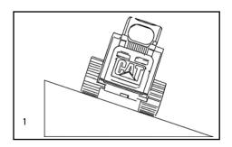
When working up and down a slope (Illus. 2), always keep the heaviest end of the machine uphill. You should also avoid unusually heavy loads and always keep loads as low as possible. Consult the Operation and Maintenance Manual for proper machine operation on slopes.
