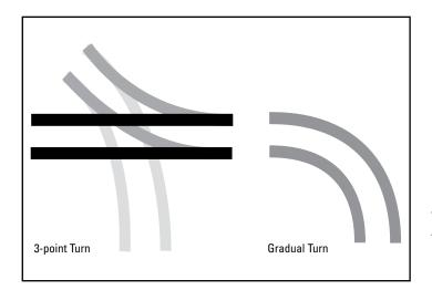
To help maximize the life of a multi terrain loader undercarriage, counter rotations should be used only when required, such as in very confined areas. Instead, use more gradual turns while slowly moving forward or in reverse. Sharp turns on abrasive material, like jagged rock, will cause premature wear to the track and roller wheels. Gradual turns will minimize cuts and tears and help maximize undercarriage component life.
