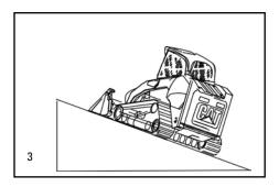
Avoid making direct 90-degree turns when operating on a slope—either on a side hill or straight up and down. Sharp turns on slopes can cause unnecessary wear on track guides (tabs) and can shove material between the track and roller wheels. In some cases, this could lead to track derailment and track damage.
