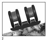
the track lugs. Uneven or excessive wear to the edge of track lugs is usually attributable to operating on slopes, and is normal.
