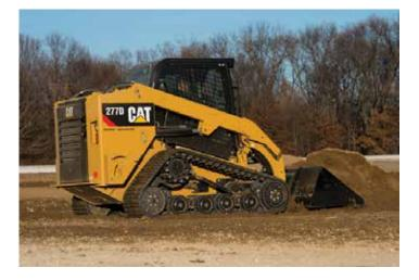
Keeping the full length of track on the ground provides the most traction and takes advantage of the machine suspension. You can get excellent results and maximize the life of your undercarriage by backdragging with loader arms in the FLOAT position. If more down pressure is needed, the suspension system on an MTL will allow for additional down pressure to be applied without raising the undercarriage off the ground. Add only the pressure required to smooth the surface.
