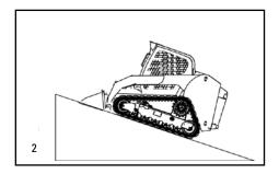
Turning when on a slope requires special attention. When turning to go DOWN a slope, first stop the machine. Then slowly turn the machine while backing down the slope (Illus. 3). When turning to go UP a hill, again, stop the machine, then turn the machine while you slowly back down the slope or until the machine is facing the desired direction of travel. Then carefully proceed forward.
