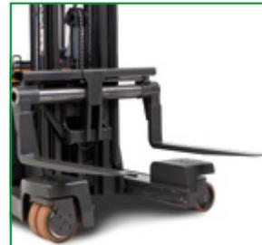
Reach out battery for easy inspection is standard. Battery on steel rollers or motor power rollers for quick one-minute change is optional.
