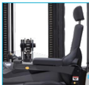
Large load wheels and brakes ensure safe handling. Synchronised steering system for quick change between normal and lateral driving is standard.
